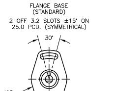
SHAFT FLAT ALIGNED WITH REFERENCE MARK IN BASE AT MID TRAVEL ±5°
