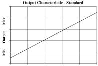
Retracted Linear Displacement Extended
