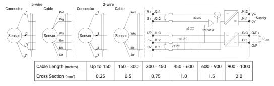
The table above shows recommended conductor sizes with respect to cable length for both three and five wire connections, based on copper conductors. Three wire connections will introduce a gain reduction of 5% and a  $\pm 1\%$  temperature dependence of gain over the range -40°C to +80°C for the cable temperature. (i.e. about -150 ppm/°C for the maximum lengths shown and less pro rata for shorter lengths.)
