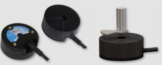
The 360° Blade Rotary Sensor accurately senses the rotary position of a metallic 'activator' mounted away from the face of the sensor. The unique non-contact two-part design utilises Gill's patented inductive technology to provide a reliable, accurate output eliminating the need for seals or bearings and ensuring long term reliability.
